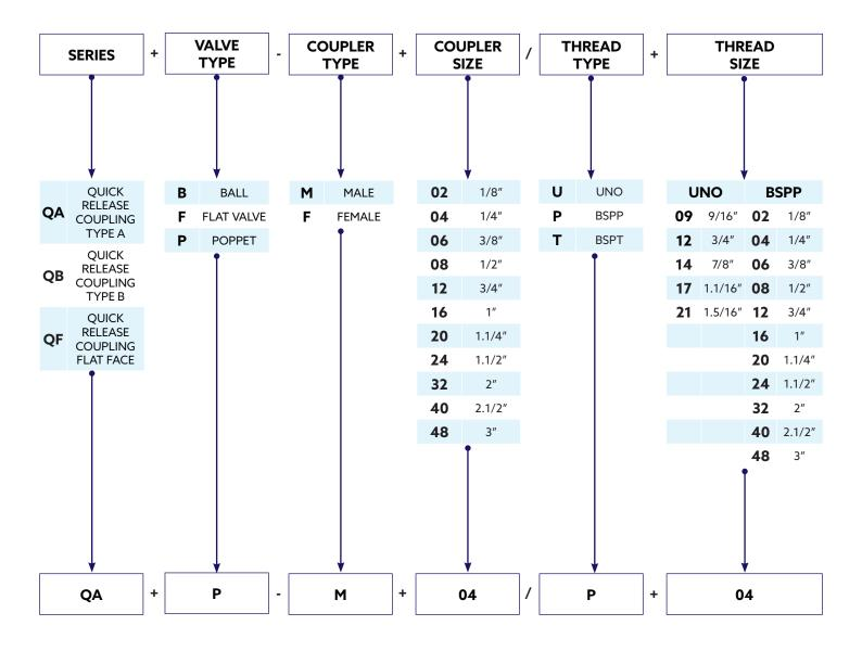
Example QAP-M04/P04 Quick Release Coupler Type A Poppet Valve 1/4" BSPP Male Tip
